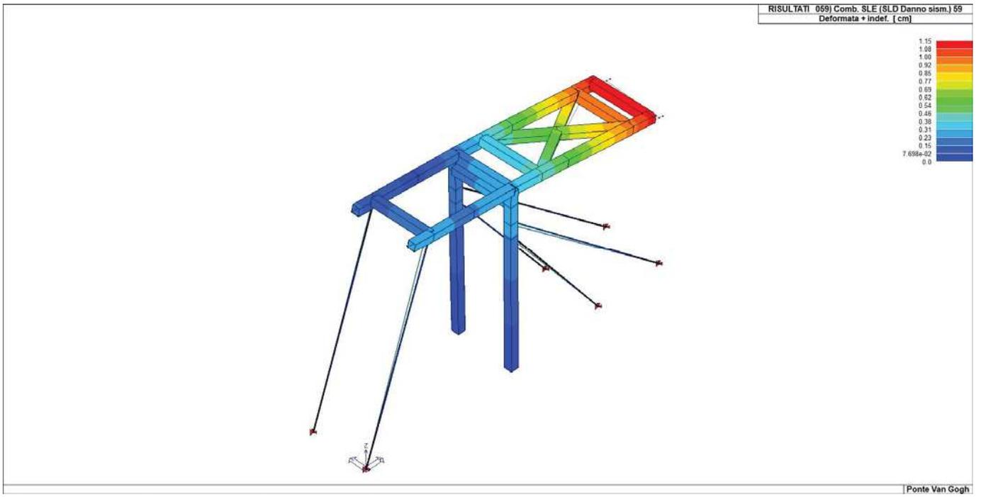
Figura 21 – Deformata massima (SLD sism.)
