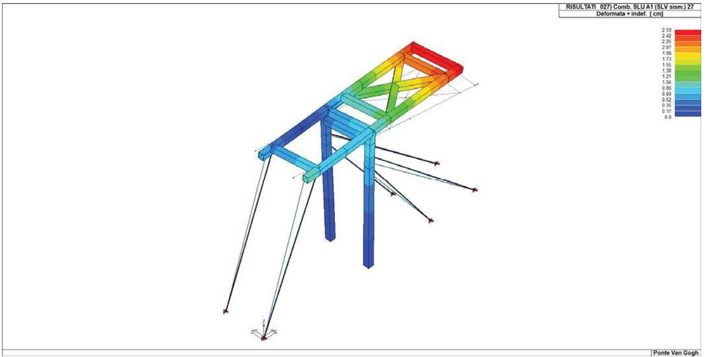
Figura 20 – Deformata massima (SLV sism.)
